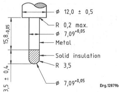
Insert the gauge as far as it will go into the guidance hole of a socket-outlet. The indicator lamp described in annex A shall light.
